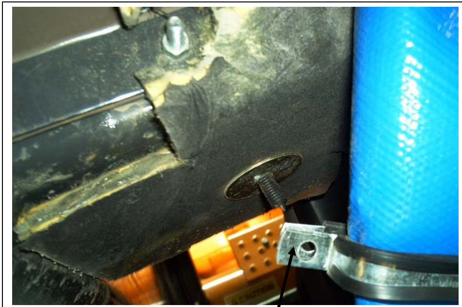
Secure hoses at this point to prevent rubbing.
