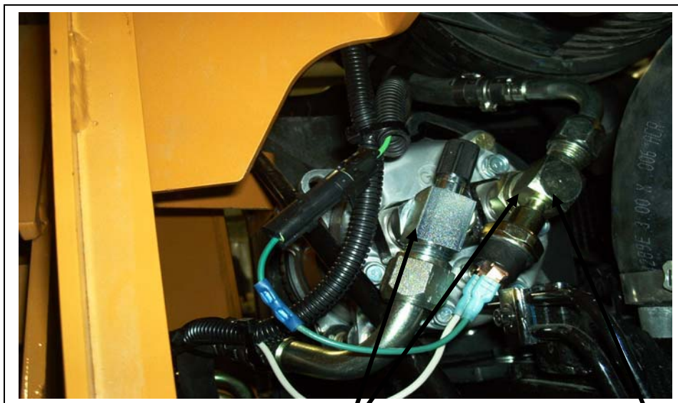
Using the nylon seal provided, install the rotolock fittings as shown.
